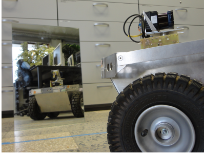
Figure 1: Robot equipped with the 3D-Hokuyo multi-echo laser scanner facing an unframed mirror.
